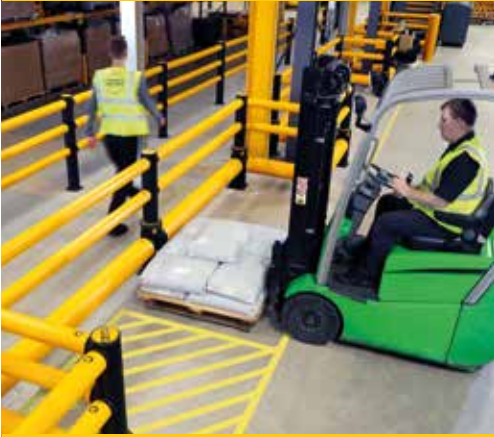
eFlex Single Traffic Barrier+ 14,400 Joules* 4 Tonne vehicle at 6mph
