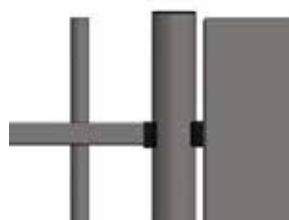
Invisible connection and inaccessible screws after installation
