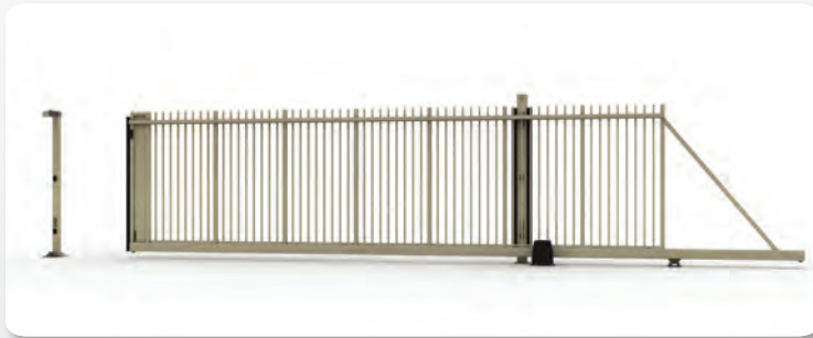
Opening: 8m - Height: 2.5m - Motor-driven operation Overstanding square bar infill
